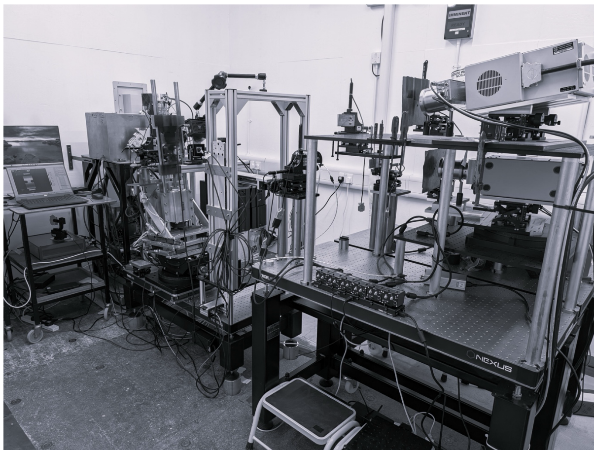
Figure S10: Photograph of the MT3.0 facility that has democratized synchrotron technology and brought combined EDXRD and 3D DIC measurement capabilities to everyday laboratory experiments.
